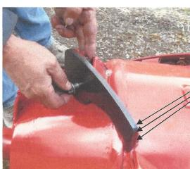
4. Fit new transition plate to backside of existing plate, aligning insert into cut out and bolt to backing plate with ½" x 2"bolt. Be sure tail end of transition plate is resting against rotor drum before tightening is completed.
